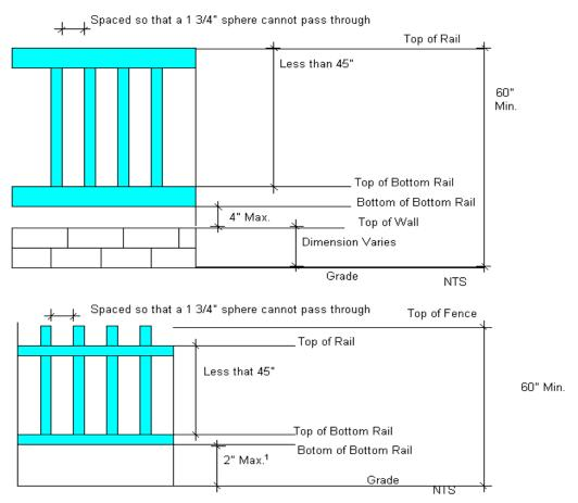
2" maximum from the grade to the bottom of the barrier may be increased to 4" maximum when grade is a solid surface such as concrete or brick paving.
