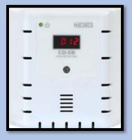
LISTEN. Leaks in CO-2 beverage dispensing systems are found using CO-2 specific sensors that are strategically placed in the building where CO-2 is used or mixed. The sensor can be part of a standalone system or wired into the building fire alarm system. The sensor and system will provide a warning signal at 1.5% (15,000 ppm) to advise that a leak has been detected and that service is needed. An evacuation signal is provided at 3% (30,000 ppm) to have the building evacuated.
