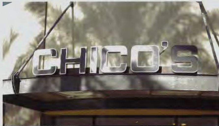
Reverse Pan Channel, Routed Face. Internally Illuminated Letters/Logo - Canopy-mounted sign application
