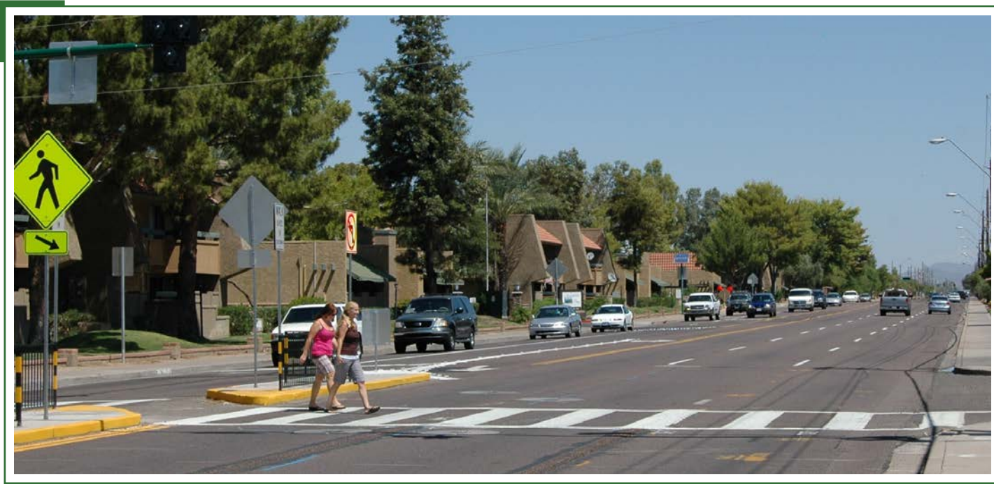
On-street facilities such as bike lanes, sidewalks, and crossing features (at intersections and midblock [pictured]) make active transportation a safe, accessible option for daily trips. Source: www.pedbikeimages.org / Mike Cynecki
