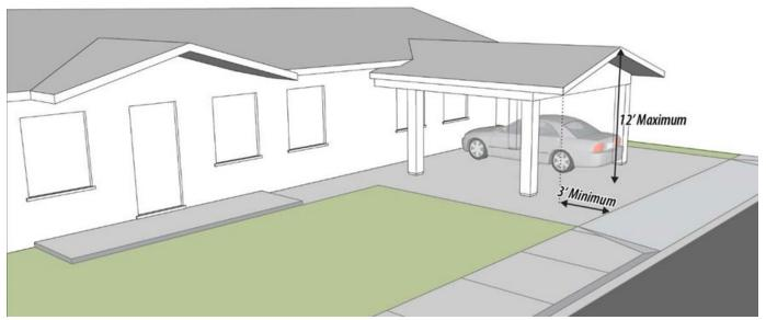
Example of an allowable shade structure. Please be aware that the right-of-way line is not always the back of the sidewalk.
