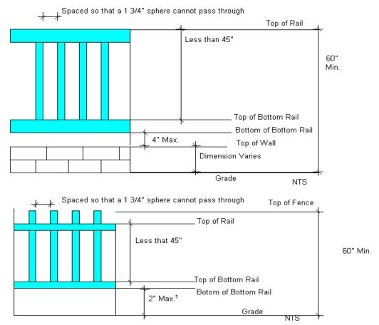
1. 2" maximum from the grade to the bottom of the barrier may be increased to 4" maximum when grade is a solid surface such as concrete or brick paving.
