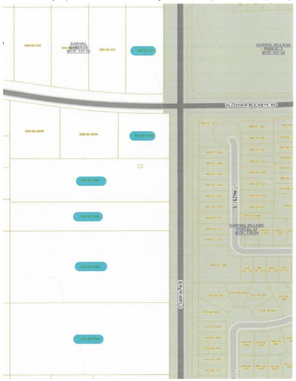
The five parcles shown below and highlighted in blue are located on the west side of Sarival Avenue. The project is needing land rights from the property owners that include right-of-way, public utility & sidewalk easements, drainage easements and temporary construction easements. All of these parcels are within the jurisdiction of Maricopa County.
